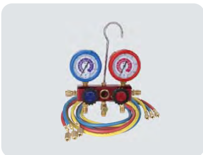
Testing manifold set for R404a,R407a,R134a and R22 manifold with 3pcs house, 2pcs qc12 quick couplers and 2pcs 2-3/4"dia.guage, 1/4"seaconnection. 3pcs 36"house.3pcs 60"house.3pcs 72"house.all house are desinged for working pressure 800psi bursting pressure 4000psi
