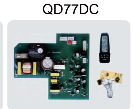
Control system for DC fan
