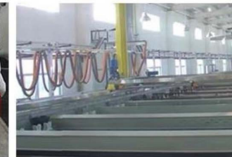
Anodizing of aluminium
